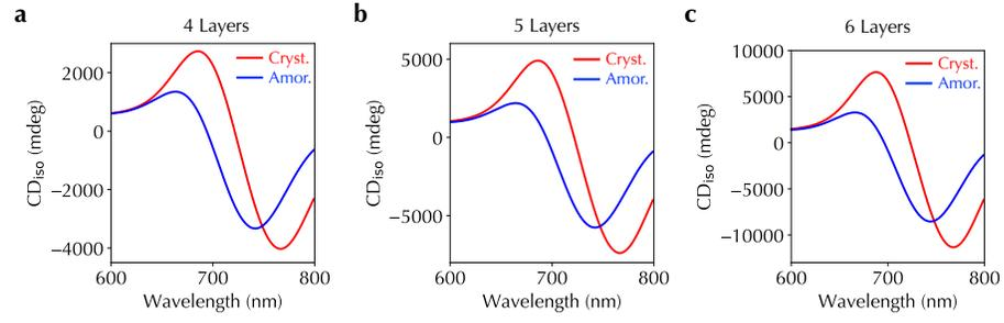
**Fig. 11** CD<sub>180</sub> spectra for heterostructures containing (a) four, (b) five, and (c) six layers of twisted aligned CNT films under GST crystalline (red lines) and amorphous (blue lines) phases.
