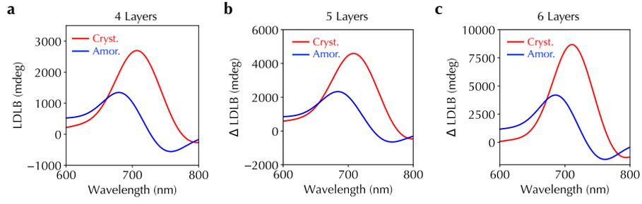
**Fig. 12** LDLB spectra for heterostructures containing (a) four, (b) five, and (c) six layers of twisted aligned CNT films under GST crystalline (red lines) and amorphous (blue lines) phases.
