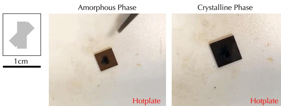
**Fig. 6** Illustration of the heterostructure sample size and photos showing the phase change on a hotplate. See Supplementary Video 1 for a full video.
