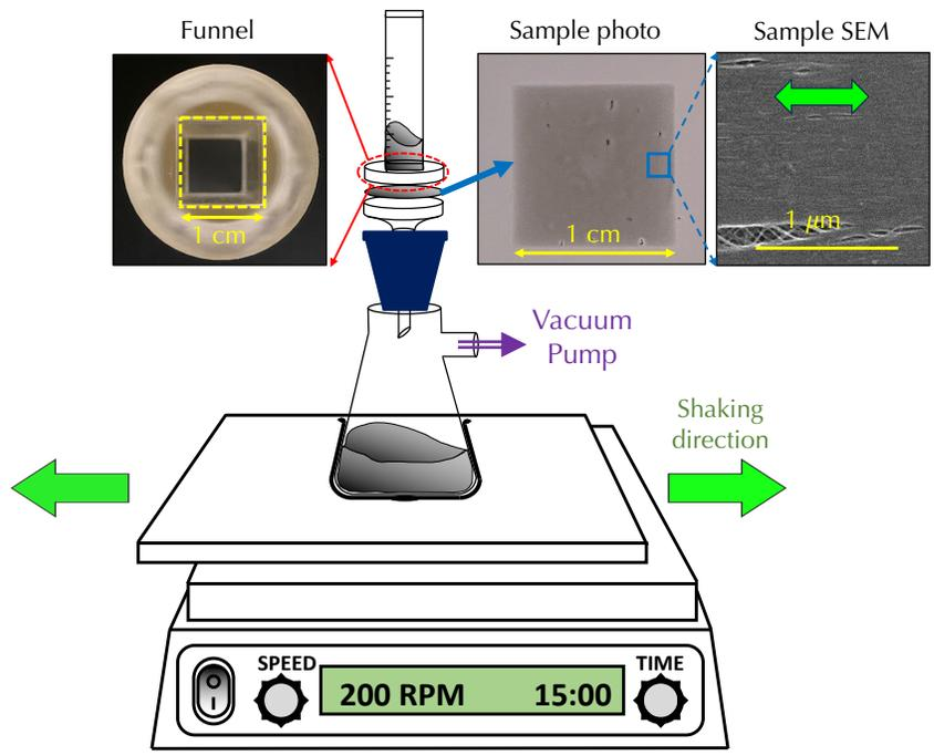
**Fig. 1** Illustration of the SAVF process, photo of a 3D-printed funnel with a square-shaped opening, photo of a fabricated square-shaped aligned CNT film, and a scanning electron microscopy (SEM) image showing alignment direction.
