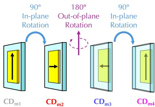
**Fig. 3** Illustration of simulating and experimentally measuring CD spectra under four sample configurations.
