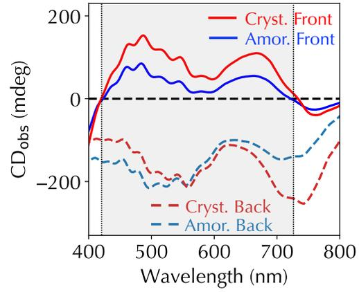
**Fig. 9** Observed CD broadband spectra measured from the front (solid lines) and back (dashed lines) sides of the same heterostructure in Fig. 3 of the main text under GST crystalline (red lines) and amorphous (blue lines) phases. The gray shaded area indicates the polarity reversal range.
