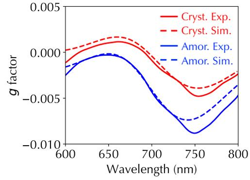
**Fig. 8** Measured (solid lines) and simulation (dashed lines) spectra of  $g$  factor under GST crystalline (red lines) and amorphous (blue lines) phases.
