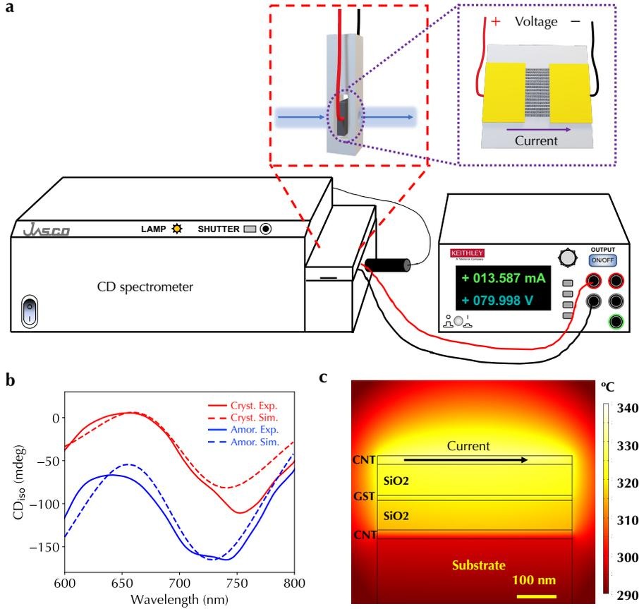
**Fig. 5 Electrical tunability of chiroptical responses in the heterostructure.** (a) Illustration of *in-situ* programming of the heterostructure in the CD spectrometer. (b) Experimentally measured (solid lines) and simulation (dashed lines)  $CD_{180}$  spectra under GST amorphous (blue lines) and crystalline (red lines) phases, respectively. (c) Spatial temperature distribution of a scaled-down heterostructure.
