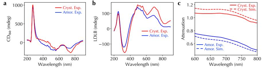
**Fig. 7** Measured broadband spectra of (a)  $CD_{180}$ , (b) LDLB, and (c) corresponding measured (solid lines) and simulation (dashed lines) average absorption spectra of LCP and RCP light under GST crystalline (red lines) and amorphous (blue lines) phases for the heterostructure in Fig. 3 of the main text.
