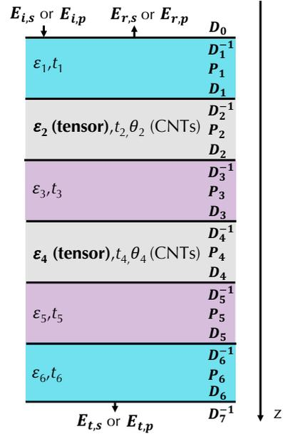
**Fig. 2** Illustration of transfer matrix method to calculate transmission and reflection coefficients of the chiroptical heterostructure containing anisotropic and isotropic materials.
