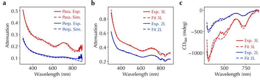
**Fig. 4** Measured (solid lines) and simulation (dashed lines) (a) linear-polarization-dependent absorption spectra under parallel polarization (red lines) and linear polarization (blue lines) for an aligned CNT film, (b) average absorption spectra of LCP and RCP light for 2-layer (blue lines) and 3-layer (red lines) twisted stacks containing only aligned CNT films, (c)  $CD_{iso}$  spectra of 2-layer (blue lines) and 3-layer (red lines) twisted stacks containing only aligned CNT films.
