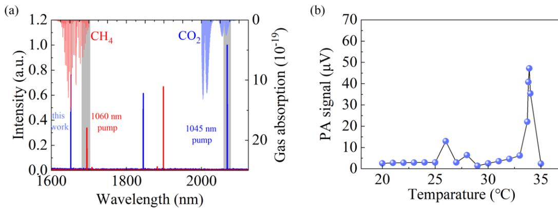
**Fig. 6** (a) Raman spectrum for dual-gas ( $\text{CH}_4/\text{CO}_2$ ) detection generated from two pump lasers. Absorption spectrum of  $\text{CH}_4$  and  $\text{CO}_2$  are from HITRAN. (b) PA signal against the seed laser temperature for  $\text{CO}_2$  detection.
