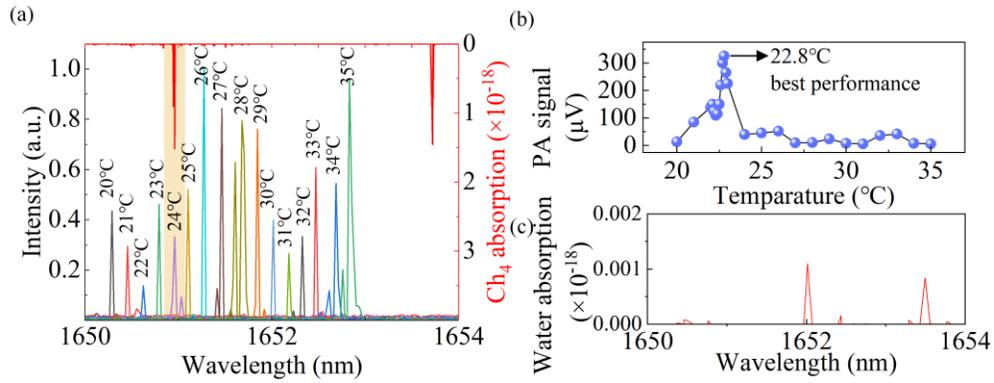
**Fig. 3** (a) Absorption spectrum of CH<sub>4</sub> (from HITRAN [29]) and laser spectra at ~1650nm at different laser temperatures. (b) PA signal against laser temperature. (c) Absorption spectrum of water (from HITRAN [29]).
