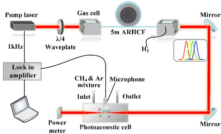
**Fig. 1** Experiment setup of the developed laser and photoacoustic system. ARHCF: anti-resonant hollow-core fiber.
