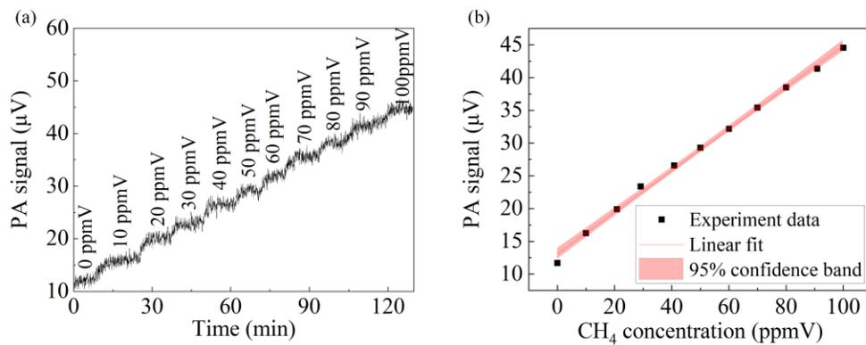
**Fig. 4** Gas detection results and system characterization. (a) Photoacoustic signal against CH<sub>4</sub> concentrations from 0 ppm to 100 ppm. (b) Linear model between photoacoustic signal and concentration.
