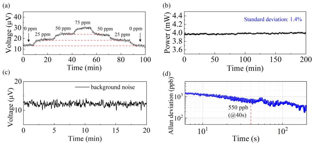
**Fig. 5 Gas detection system characterization.** (a) Repeatability of gas detection within 100 minutes. (b) Power monitoring of beam after photoacoustic gas cell with pure Ar within 200 minutes. (c) Background noise signal recorded with pure Ar within 20 minutes. (d) Allan deviation of background signal in (c).
