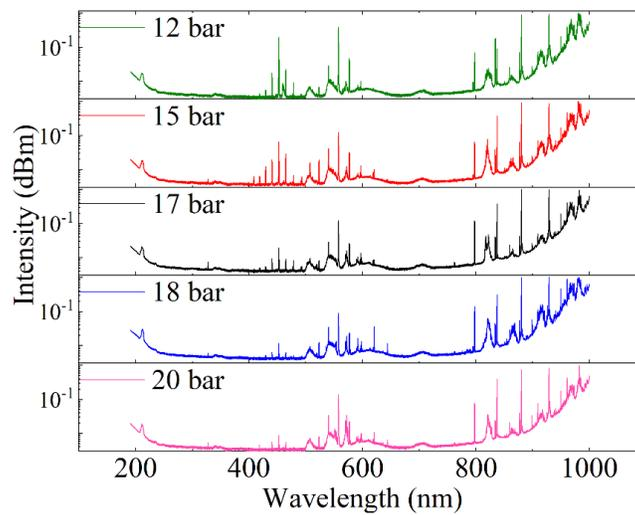
**Fig. 7** Spectrum evolution of wavelength range less than 1  $\mu\text{m}$  at different gas pressure.
