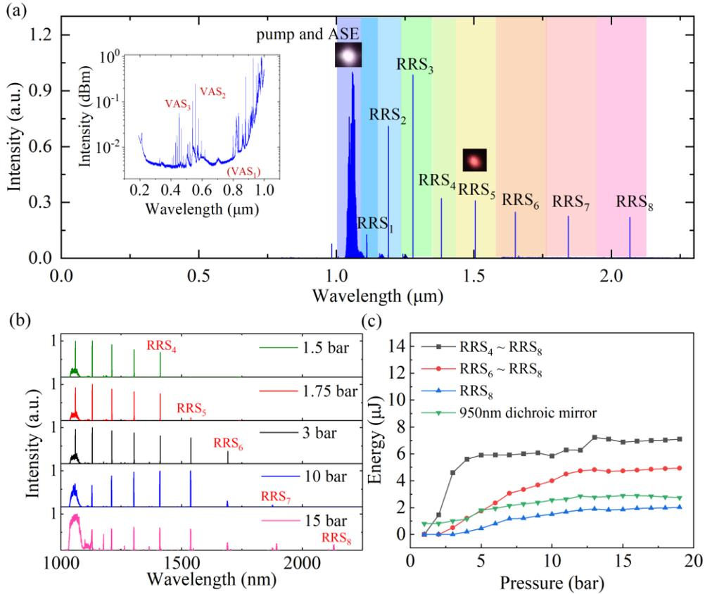
**Fig. 2.** (a) Spectrum from UV to NIR and spots of Raman lines. (b) Spectrum evolution of NIR wavelength at 1.5 bar, 1.75 bar, 3 bar, 10 bar, and 15 bar pressure. (c) Pulse energy of Raman laser against H<sub>2</sub> pressure.
