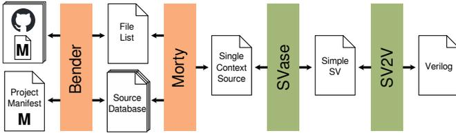
Fig. 2. Basilisk’s SV-to-Verilog RTL description preprocessing flow.
