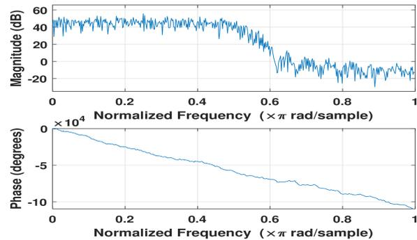
(b) Received signal with CAZAC code as preamble after CFO Compensation
