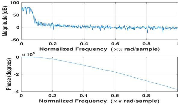
(a) Received signal with Golay code as preamble after applying filter
