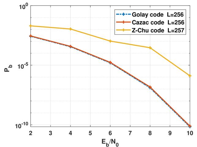
Figure 4: Probability of error VS  $E_b/N_0$  for different preamble sequences
