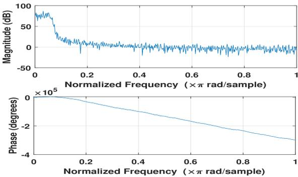
(a) Received signal with CAZAC code as preamble after applying filter
