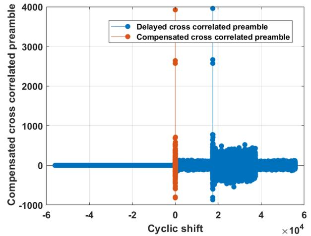
Figure 7: Cross correlation of transmitted and received preamble for CAZAC code SNR=8dB, preamble length=64
