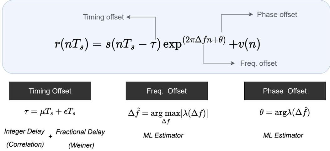
Figure 1: Synchronization and offsets in received signals [9]
