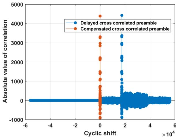
Figure 6: Cross correlation of transmitted and received preamble for Golay code SNR=8dB, preamble length=64
