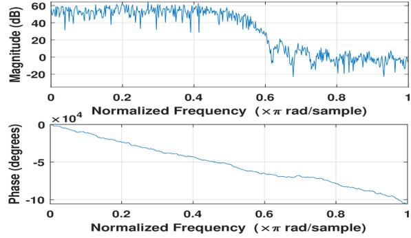
(b) Received signal with Golay code as preamble after CFO Compensation
