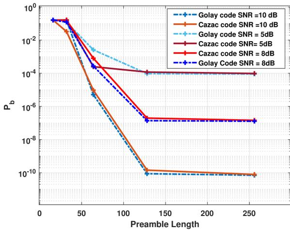
Figure 5: Comparison of Preamble sequences for varying  $E_b/N_0$
