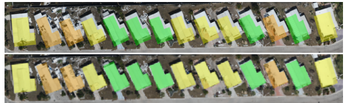
Fig. 5: An example of spatial alignment error correction with the vector fields generated through the process described in [40]. [Top] The raw, unaligned, building polygons (colored in green, yellow, and orange) sourced from Microsoft Building Footprints [3] overlaid over the geospatial imagery. [Bottom] The aligned building polygons (colored in green, yellow, and orange) derived from the generated vector fields from adjustment annotations. Note the difference in overlap in building polygons and the buildings within the imagery.
