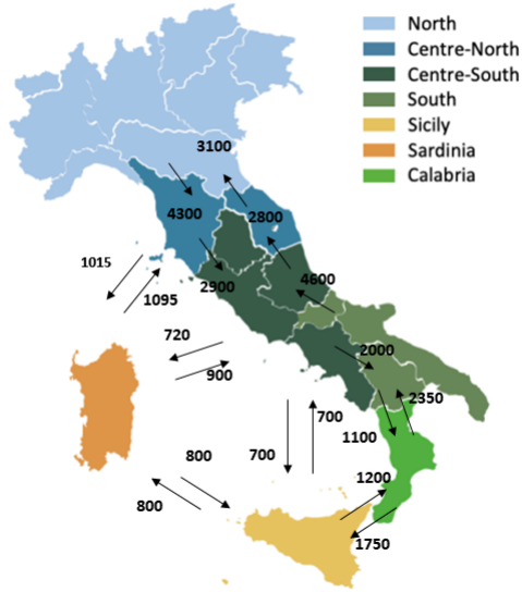
Figure 15: Representation of the spatial resolution of the Italian power model. The seven nodes of the model aggregate different Italian regions, according to the colours in the picture. The zones are linked through high-voltage power lines, whose transmission capacity is indicated with the values in the graph [GW]. The capacity values assume that the already announced grid expansion projects up until 2026 are built [87].
