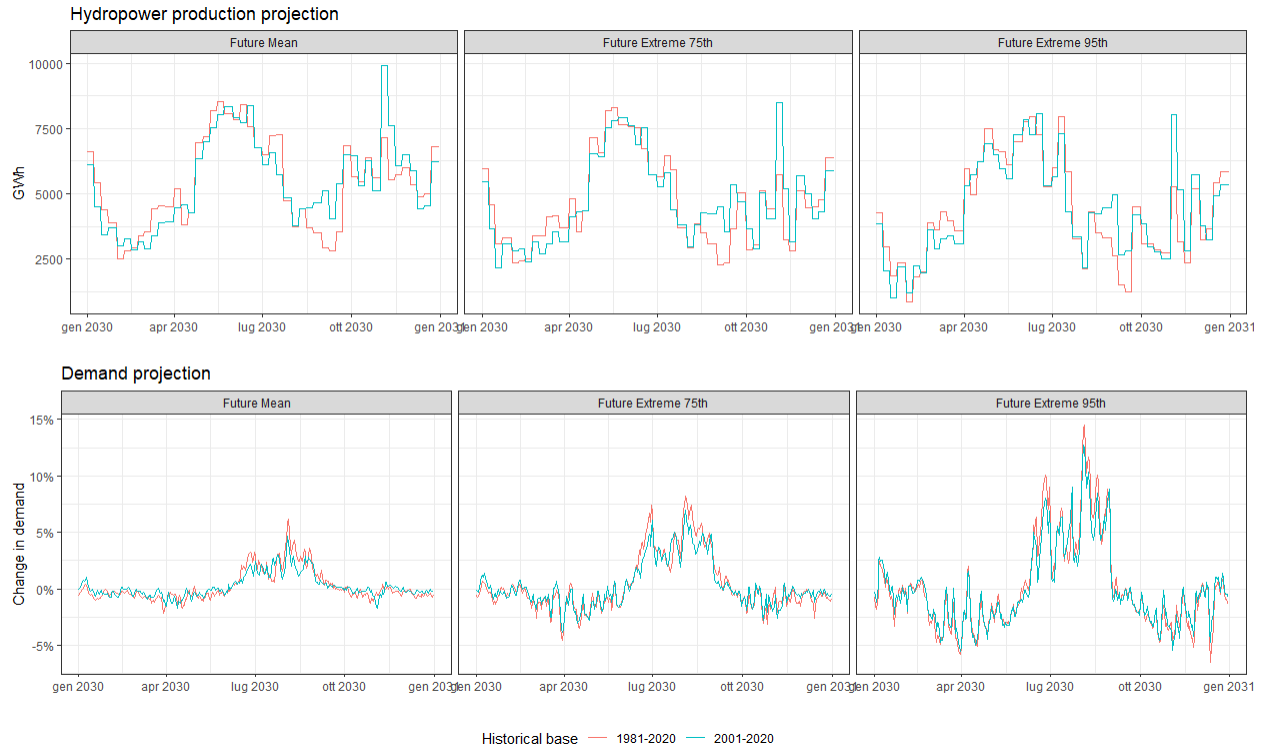
Figure 13: Comparison of input projections of hydro production and electricity demand change, by choice of historical base year period
