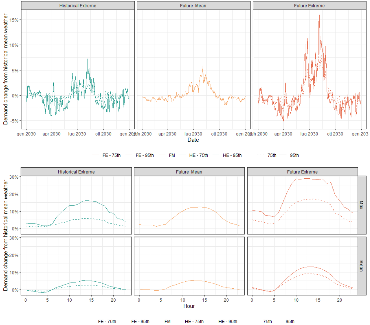
Figure 1: Climate change impacts on electricity demand. Panel above: Changes in daily load with respect to the mean weather scenario, in each alternative climate scenario. Panel below: Changes in hourly load in the summer with respect to the mean weather scenario, in each alternative climate scenario. Solid lines show the change of the 95th percentile, while dashed lines of the 75th percentile.
