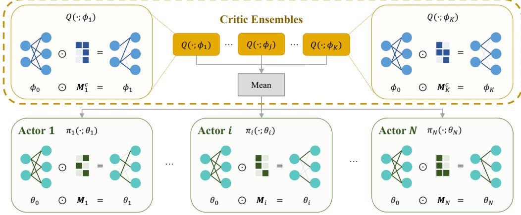
Figure 2: Overall network architecture of Kaleidoscope. It maintains one set of parameters  $\theta_0$  with  $N$  sets of masks  $[\mathbf{M}_i]_{i=1}^N$  for actor networks, and one set of parameters  $\phi_0$  with  $K$  sets of masks  $[\mathbf{M}_j^c]_{j=1}^K$  for critic ensemble networks, where  $N$  is the number of agents,  $K$  is the number of ensembles, and  $\odot$  denotes the Hadamard product.
