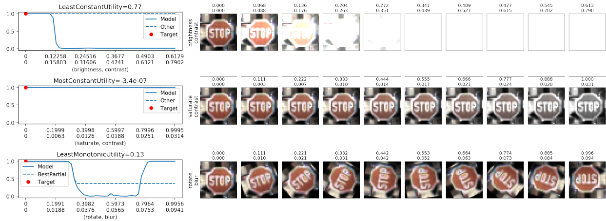
Figure 6: The dependence plots for traffic sign detection show which transformation is the most sensitive (top), the least sensitive (middle), and the least monotonic (bottom). These curves highlight both expected model trends (top) and unexpected trends (middle and bottom), where the model seems to ignore color and fails when the stop is rotated partially but works again when the stop sign is almost flipped over.
