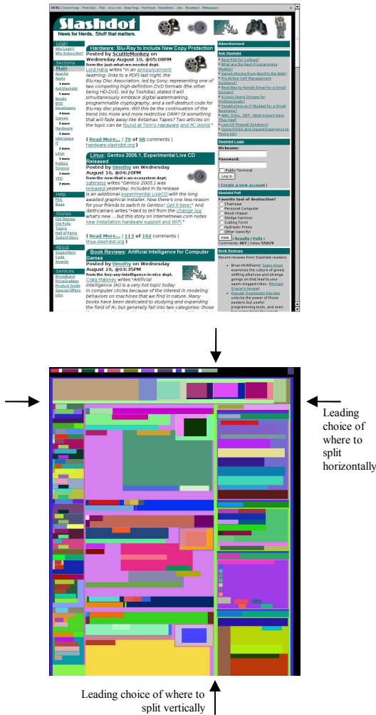
Figure 4: The Slashdot ( http://slashdot.org ) web page and an extracted DOM representation (bottom) (note that major DOM elements shown for clarity). The colors in the DOM element are randomly chosen to demarcate the different DOM elements found. The arrows on the left and right are the leading choice of places to split horizontally. The arrows on the top and bottom of the DOM are the leading choices, based on entropy, of where to split the page with a vertical cut. Note that some of the DOM elements (for example at the top) will be cut.
