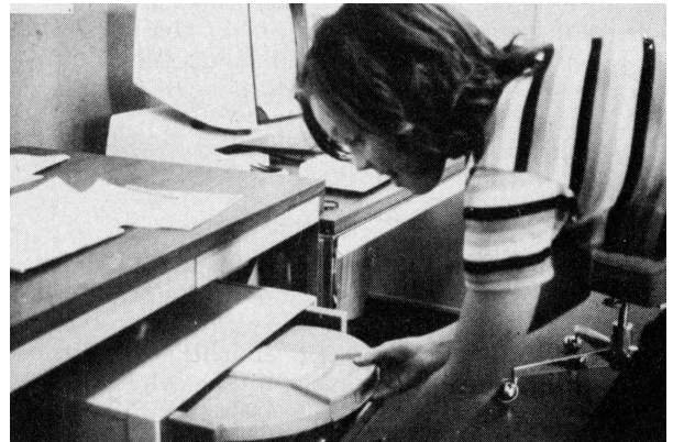
Figure 26.4. Inserting the disk pack in the Dynabook.
