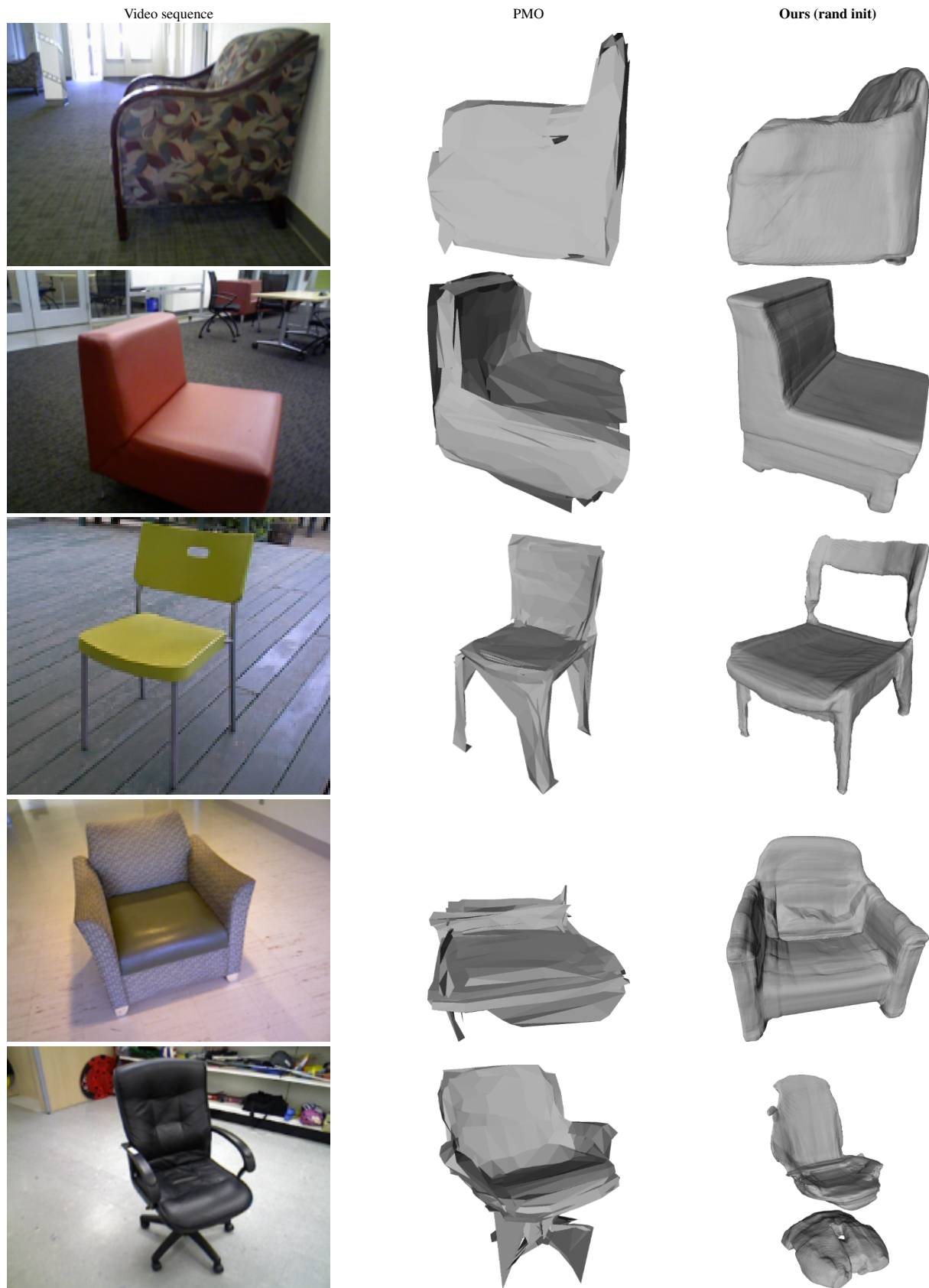
Figure 12. More Comparisons on 3D shape prediction from multi-view images on real-world chair dataset [1]. It is in general challenging for shape prediction on real images. Comparatively, our method produces more reasonable results with correct structure.
