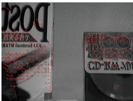
Figure 5. Result of the detected optical flow
