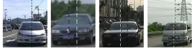
Figure.2 Examples for the symmetry axes. White dashed represents gray symmetry axis; Black dashed represents binary value symmetry axis; Dash-dot represents S component symmetry axis
