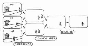
Fig. 4 A Method to Extract Moving Objects
