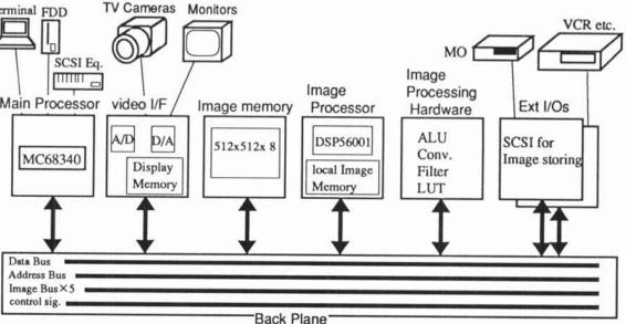
Fig. 8 Hardware Block Diagram of Proto-type System
