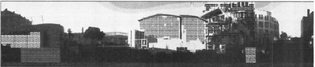
Fig.7(b) Example of planar face extraction result Planar faces are represented by the laser range points belonging to them, different planar faces are given different intensity values.
