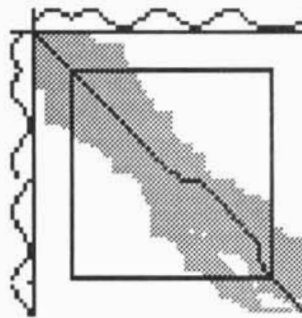
Figure 2. Parallel paths development when comparing 2 lines/columns (shaded area ; bold path gives the minimal cost path for compared signals).
