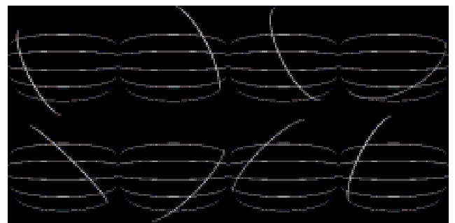
Fig.5 Slit images of the sphere projected by Pentagramma and a freehand light stripe
