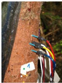
Figure 1: Sap flow measurement by heat field deformation method (Nadezhdina et al. 1998).
