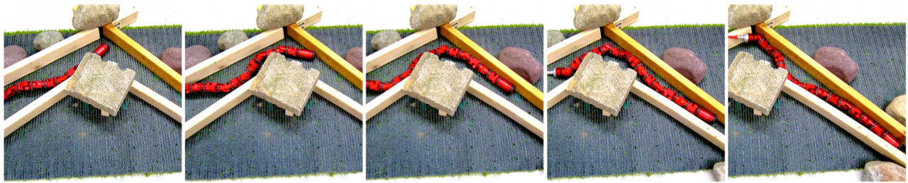
Fig. 8: A montage of the robot undergoing the a low-impedance slithering gait. The robot executes the gait cycle and progress forward, but can be easily deformed from the nominal shape. This allows the robot to progress around a bend that would not have been possible with a standard position-controlled gait.
