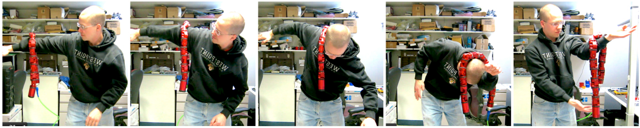
Fig. 6: A montage of the robot undergoing the compliant roll-in-shape motion. The robot actively rolls along while compliantly adapting its shape to match its surroundings.
