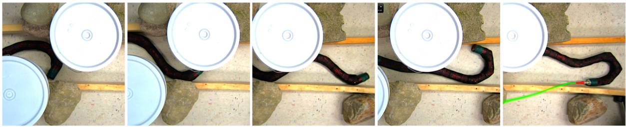
Fig. 10: A montage of the low-impedance sliding motion, with an open-loop head oscillation to initiate motion. The robot undulates until the shape of the robot closely matches the shapes of the buckets and the snake slides through. Afterwards, the head continues to oscillate, causing the robot to turn in place.
