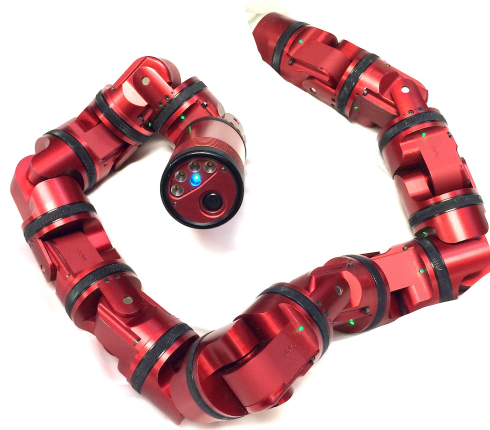
Fig. 1: A photo of the Series Elastic Actuated Snake robot ( SEA Snake ). Each module of the robot has series elastic actuation that enables compliant motion and torque sensing.
