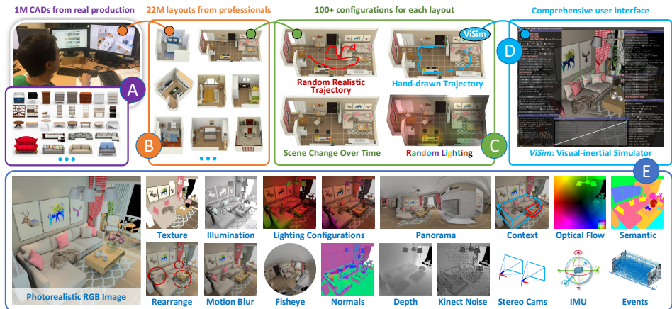
Figure 2: System Overview: an end-to-end pipeline to render an RGB-D-inertial benchmark for large scale interior scene understanding and mapping. (A) We collect around 1 million CAD furniture models from world-leading furniture manufacturers. These models have been used in the real-world production. (B) Based on those models, around 1,100 professional designers/companies create around 22 million interior layouts. Most of such layouts have been used in real-world decorations. (C) For each layout, we generate a number of configurations to represent different lightings and simulate scene change over time in daily life. (D) We provide an interactive simulator ( ViSim ) to create the ground truth monocular/stereo trajectories, as well as IMU and event camera data. Trajectories can be set manually, or using random walk and neural network based generation. (E) All supported image sequences and ground truth data.
