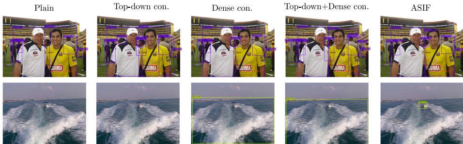
Figure 5: Qualitative results of different methods. The first row demonstrates the detection when objects are occluded by others. The second row shows results when an object appears in the ambiguous background (the water ripple looks like a deck).
