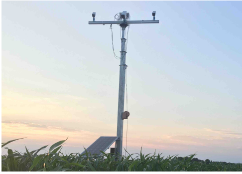
Figure 1: Mobile Observation Tower with two RGB cameras and a thermal camera in between
