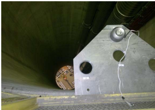
Figure 3 : Adapted Taylor Hobson sphere and forced centring plate above the ECA4 shaft
