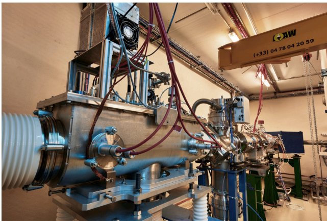
Fig. 5. The RFQcb installed at the Offline 2 facility (looking upstream to the separator magnet) [Cern Document Server 2690229].
