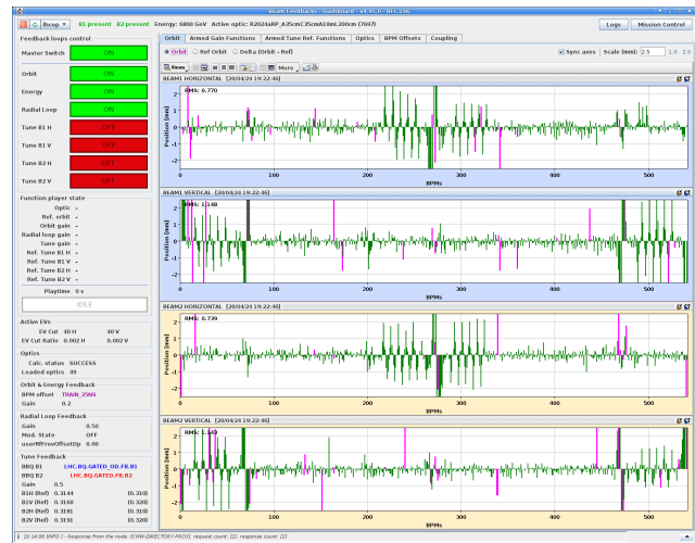
Figure 2: OFB Dashboard application used daily in LHC operation with BPM readings.
