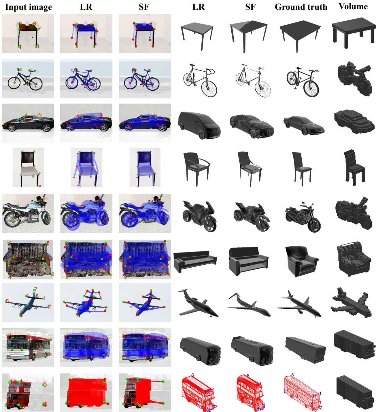
Figure 6. Visual evaluation of estimated 3D models by our proposed methods for eight object categories including diningtable, bicycle, car, chair, motorbike, sofa, aeroplane, and bus. We denote green nodes as labelled landmarks, red nodes as projected landmarks, and red number as landmarks index. The columns here shows respectively (1) the input images with landmarks and silhouette, (2) projection of dense model estimated by landmark registration, (3) projection of dense model estimated by silhouette fitting with all components, (4) the dense model estimated by landmark registration, (5) the dense model estimated by silhouette fitting with all components, (6) ground truth, and (7) volumetric representation of ground truth. The failure case is shown in red in the last row. Best viewed in color.
