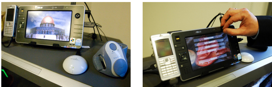
Figure 2. The central module of our AAL system on top of a television set showing family photos when not in use (left), and becoming active when touched (right)
