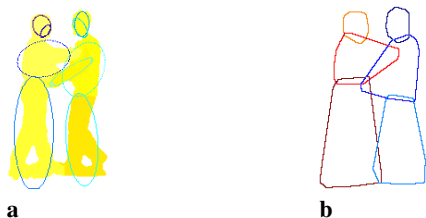
Fig. 3. Body-part parameterization for Fig. 1b. Each body part is parameterized by both an ellipse (a) and a convex hull (b)
