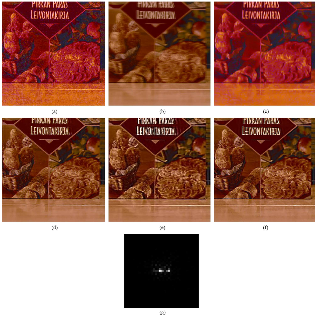
Fig. 9. Real image example (courtesy of [17]). (a) Short exposure image, (b) long exposure image, (c) denoised short exposure image, (d) restored image using [17], (e) restored image using the algorithm [4], (f) restored image using the proposed algorithm, and (g) recovered PSF using the proposed algorithm (support : 41 \times 41 ).
