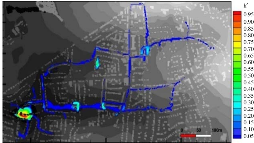
Fig. 6: Flood map of central model (West Garforth case study area) showing water depth h in meters
