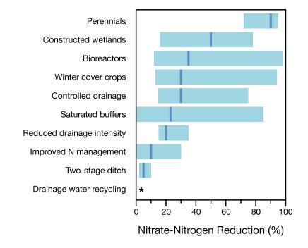
\*Drainage water recycling: Although research results have been promising, this is a new practice for which greater understanding of design and management is required before nitrogen reduction effectiveness can be calculated.
