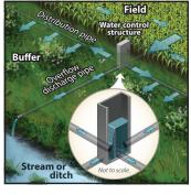
a drain outlets through a buffer that is at a lower elevation than the field. Soil must contain high organic matter content and not have layers of high permeability (sand or gravel layers).
