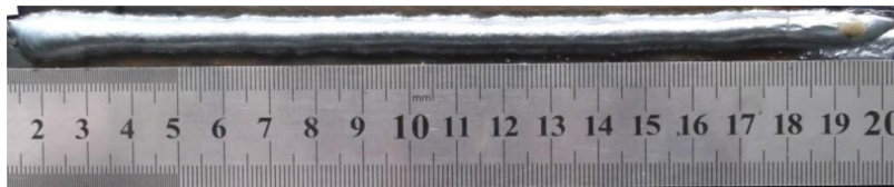
Fig. 13. Welding seam of experiment 9.
