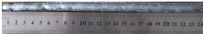
Fig. 6. Welding seam when the transition phase is not employed.
