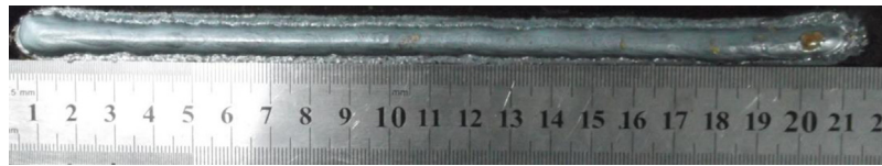
Fig. 8. Welding seam when the transition phase is employed.
