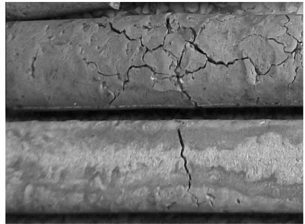
Fig. 5. Macro-cracks in specimens under sulfate attack.
