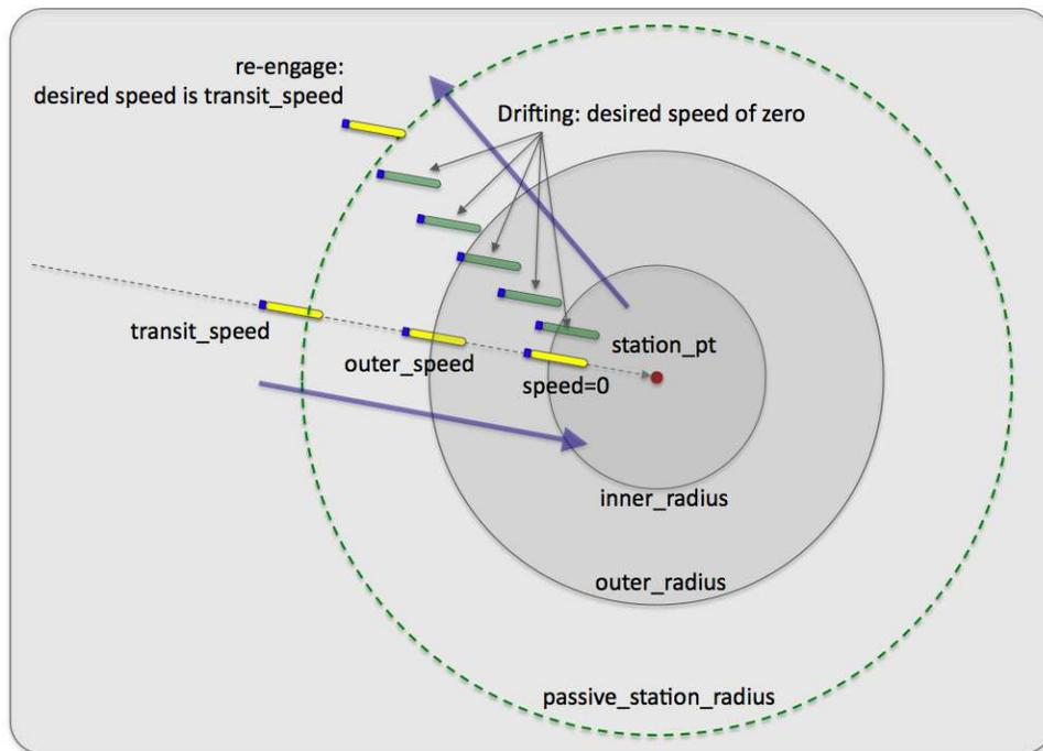
Figure 47: **Passive station-keeping:** The station-keep behavior can be configured in the “passive” mode. The vehicle will move toward the station point until it reaches the `inner_radius` or until progress ceases. It will then drift until its distance to the station point is beyond the `passive_station_radius`. At this point it will re-engage to reach the station-point and may trigger another behavior to dive.
