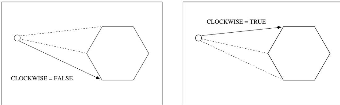
Figure 40: In the *acquire* mode, the polygon points are evaluated for suitability in terms of a smooth entry trajectory. Only the “viewable” points, those viewable if the polygon were an opaque object and the viewer were at the current vehicle location, are contenders. The contenders are rated on the follow-on angle given the desired clockwise or counter-clockwise loiter direction. Larger follow-on angles are preferred as shown.
