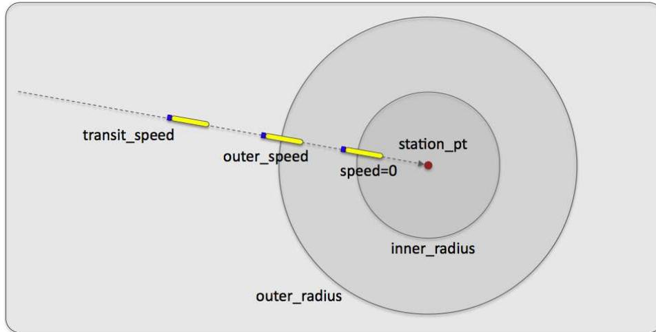
Figure 46: **The station-keep behavior parameters:** The station-keep behavior can be configured to approach the outer station circle with a given transit speed, and will decrease its preference for speed linearly between the outer radius and inner radius. The preferred speed is zero when the vehicle is at or inside the inner radius.
