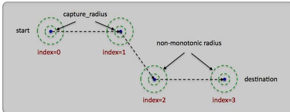
Figure 35: **The BHV\_Waypoint behavior:** The waypoint behavior basic purpose is to traverse a set of waypoints. A capture radius is specified to define what it means to have achieved a waypoint, and a non-monotonic radius is specified to define what it means to be "close enough" should progress toward the waypoint be noted to degrade.
