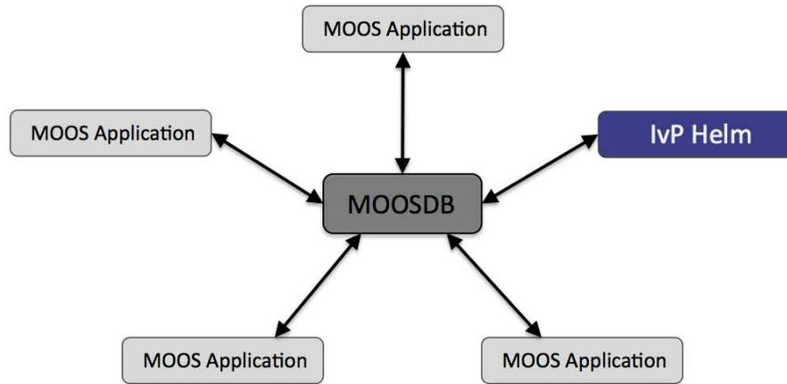
Figure 3: **A MOOS community:** is a collection of MOOS applications typically running on a single machine each with a separate process ID. Each process communicates through a single MOOS database process (the MOOSDB) in a publish-subscribe manner. Each process may be executing its inner-loop at a frequency independent from one another and set by the user. Processes may be all run on the same computer or distributed across a network.
