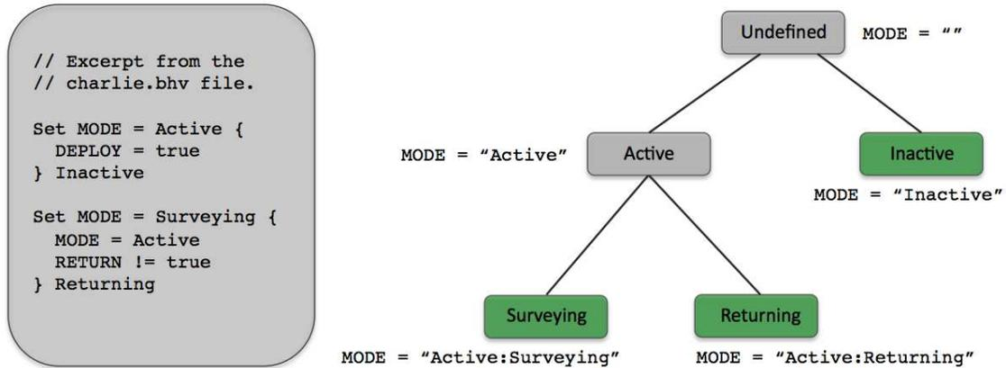
Figure 12: **Hierarchical modes for the Charlie mission:** The vehicle will always be in one of the modes represented by a leaf node. A behavior may be associated with any node in the tree. If a behavior is associated with an internal node, it is also associated with all its children.
