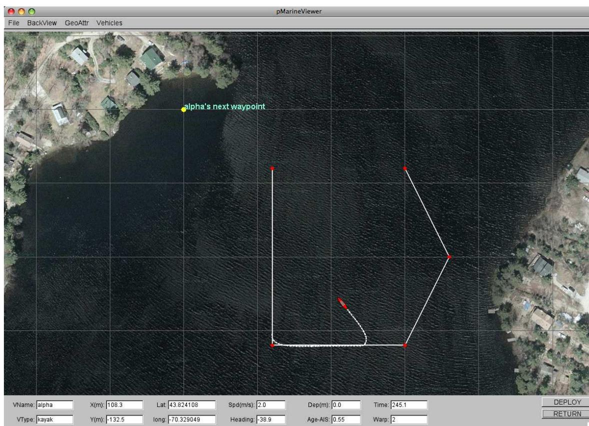
Figure 7: **The Alpha Example Mission - In the Returning Mode**: The vehicle can be commanded to return prior to the completion of its waypoints by the user clicking the **RETURN** button on the viewer.
