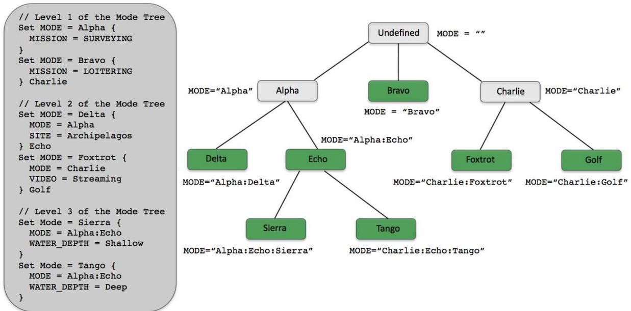
Figure 13: **Example Hierarchical Mode Declaration:** The hierarchy on the right is constructed from the set of mode declarations on the left (with fictional conditions). Darker nodes represent modes that are realizable through some combination of conditions.
