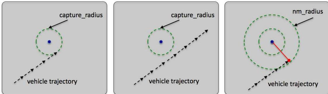
Figure 36: **The capture radius and non-monotonic radius:** (a) a successful waypoint arrival by achieving proximity less than the capture radius. (b) a missed waypoint likely resulting in the vehicle looping back to try again. (c) a missed waypoint but arrival declared anyway when the distance to the waypoint begins to increase and the vehicle is within the non-monotonic radius.
