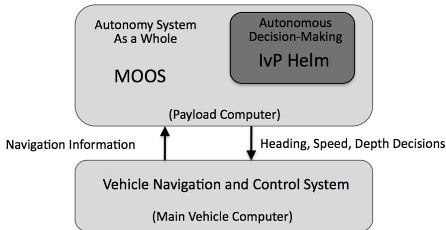
Figure 2: **The backseat driver paradigm:** The key idea is the separation of vehicle autonomy from vehicle control. The autonomy system provides heading, speed and depth commands to the vehicle control system. The vehicle control system executes the control and passes navigation information, e.g., position, heading and speed, to the autonomy system. The backseat paradigm is agnostic regarding how the autonomy system implemented, but in this figure the MOOS-IvP autonomy architecture is depicted.
