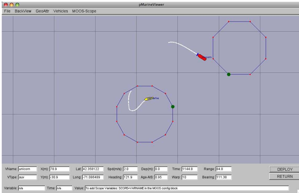
Figure 24: A screen shot of the pMarineViewer application running with two vehicles - one kayak platform, and one AUV platform. The charlie kayak platform is the *active* platform meaning the data fields on the bottom reflect the data for this platform.
