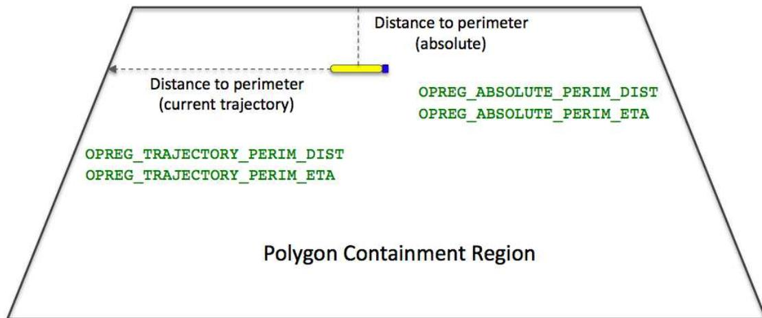
Figure 39: **The OpRegion polygon and status variables:** The OpRegion behavior publishes information regarding its estimated distance and time of arrival (ETA) to the perimeter of the polygon containment region. It publishes two sets of information; one based on the current trajectory and the other based on the absolute distance to the perimeter at top vehicle speed.
