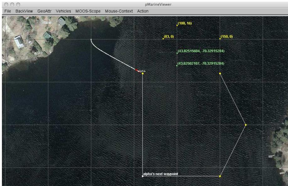
Figure 33: **Drop points:** A user may leave drop points with coordinates on the geo portion of the pMarineViewer window. The points may be rendered in local coordinates or in lat/lon coordinates. The points are added by clicking the left mouse button while holding the **SHIFT** key or **CTRL** key. The rendering of points may be toggled on/off, cleared in their entirety, or reduced by popping the last dropped point.
