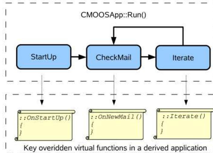
Figure 5: **Key virtual functions of the MOOS application base class:** The flow of execution once `Run()` has been called on a class derived from `CMOOSApp`. The scrolls indicate where users of the functionality of `CMOOSApp` will be writing new code that implements whatever it is that is wanted from the new applications.
