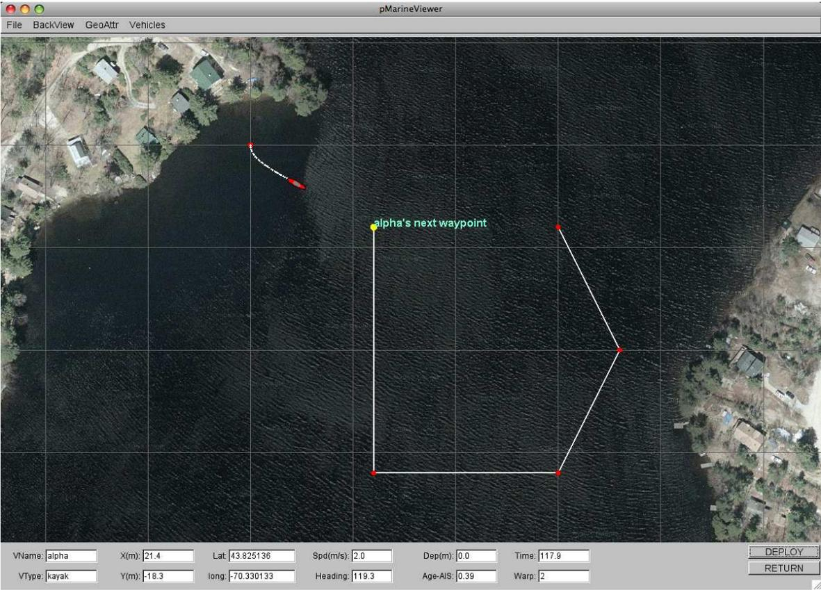
Figure 6: **The Alpha Example Mission - In the Surveying Mode**: A single vehicle is dispatched to traverse a set of waypoints and, upon completion, traverse to the waypoint (0,0) which is the launch point.
