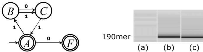
Figure 3: (Left:) A 4-states automaton used for this experiment. (Right:) The results of electrophoresis are displayed in gel-like image. Lane (a) is for the input string 1101, lane (b) for 1110, and lane (c) for 1010. Since the full-length band (190 mer) is detected in lane (b) and (c), we determine the automaton accepts two input strings (b) 1110 and (c) 1010.
