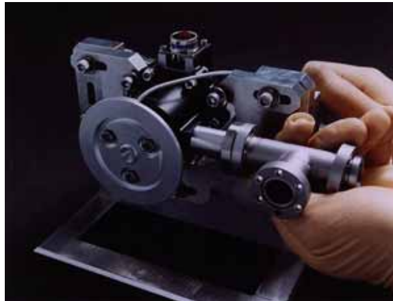
Figure 3-12. GP_B proportional micro thruster assembly
