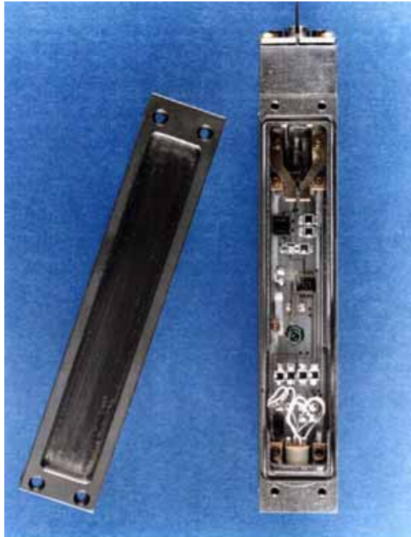
A SQUID (Superconducting Quantum Interference Device)
