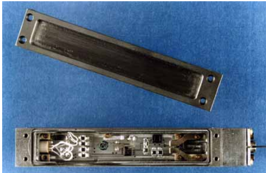
Figure 3-2. SQUID detector package, with housing cover
