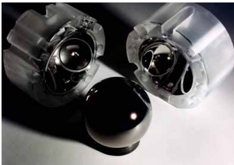
Figure 3-1. Gravity Probe B gyroscope rotor, with quartz housing halves.
