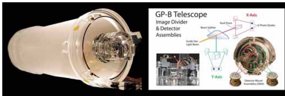
Figure 1-6. A pre-flight prototype of the GP-B telescope and diagram of its image-centering operation
