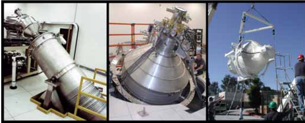
Figure 6-5. Left: Engineering Development Dewar (EDD); Middle & Right: Science Mission Dewar (SMD).
