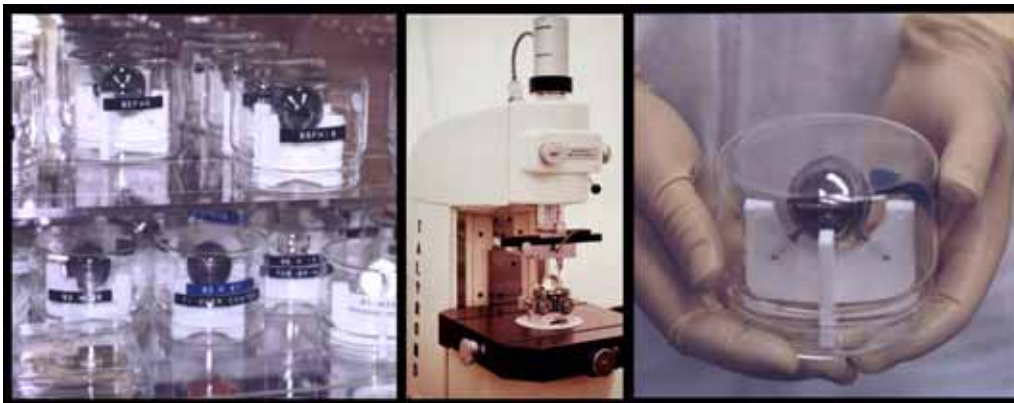
Figure 6-6. Gyroscope rotor development and precision sphericity measurement.
