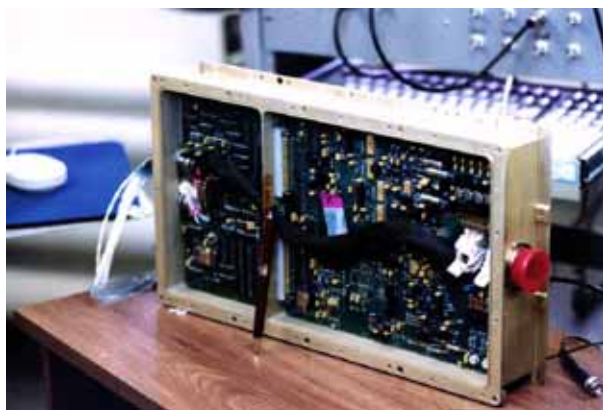
A SQUID Readout Electronics (SRE) box. Each SRE box controls four SQUID magnetometers.
