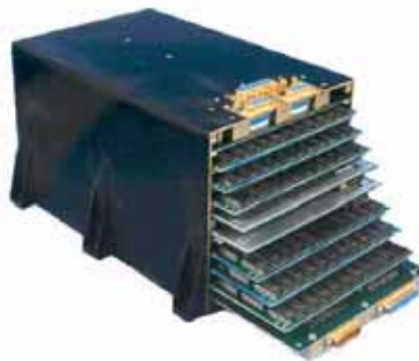
A typical solid state recorder, manufactured by SEAKR Engineering
