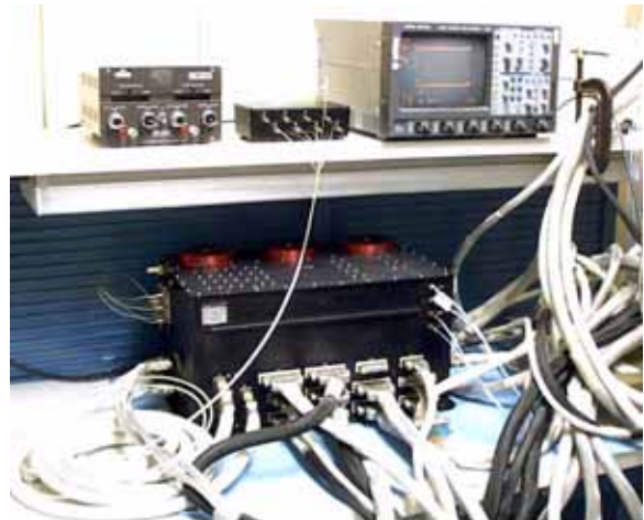
The Experiment Control Unit (ECU) box on a test bench at Lockheed Martin Corp.
