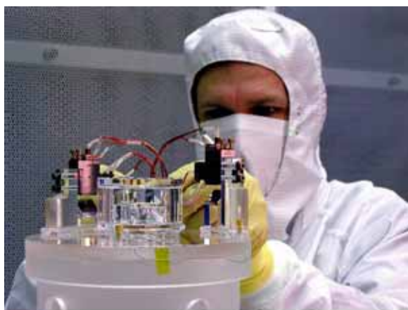
Close-up of GP-B telescope specialist, Ken Bower, adjusting the wires on the GP-B pre-flight telescope.
