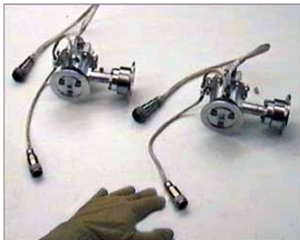
Figure 3-6. Proportional micro thrusters used for GP-B spacecraft attitude control
