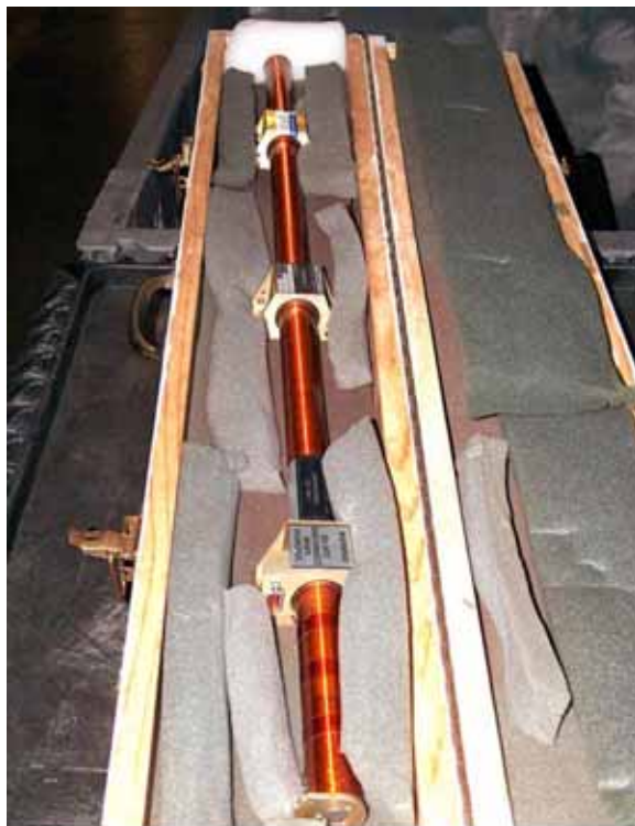
A spare GP-B magnetic torque rod. These rods are basically electromagnets located on the spacecraft frame that interact with Earth's magnetic field to control the spacecraft's orientation in orbit.
