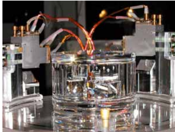
Figure 3-17. The telescope Image Divider Assembly (IDA) and Detector Package Assemblies (DPA)
