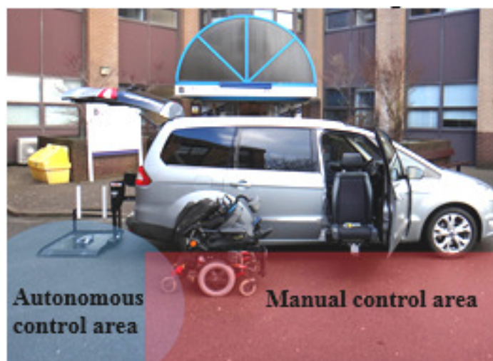
Figure 1: Autonomous docking of a powerchair using ATRS
