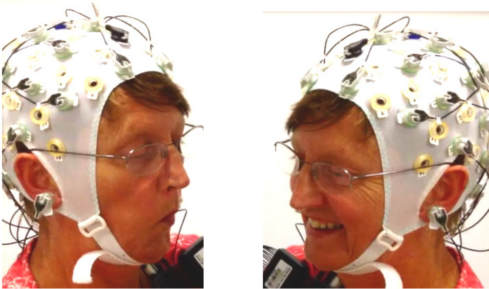
Figure 27: Participant performing tongue and mouth movements whilst wearing an actiCAP
