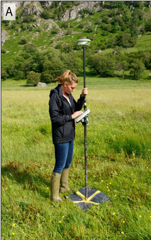
295 Figure 2 Fieldwork procedure for students to acquire aerial images: (A) RTK-GPS survey of a 296 ground target; (B) Operation of the remote control for a DJI Phantom UAV. Note that these 297 photographs were taken during undergraduate fieldwork in the UK rather than during the 298 New Zealand fieldtrip but they illustrate the same procedure.
