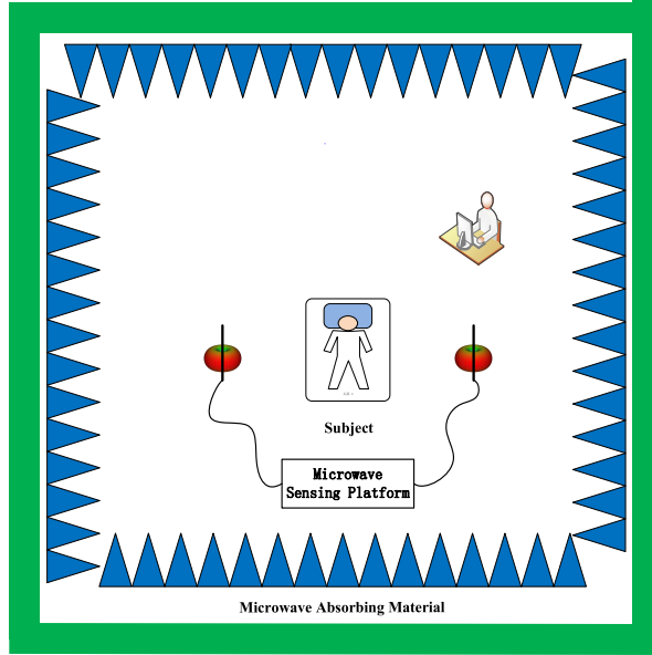
Figure 1–Experiment setup for detecting sleep apnea.
