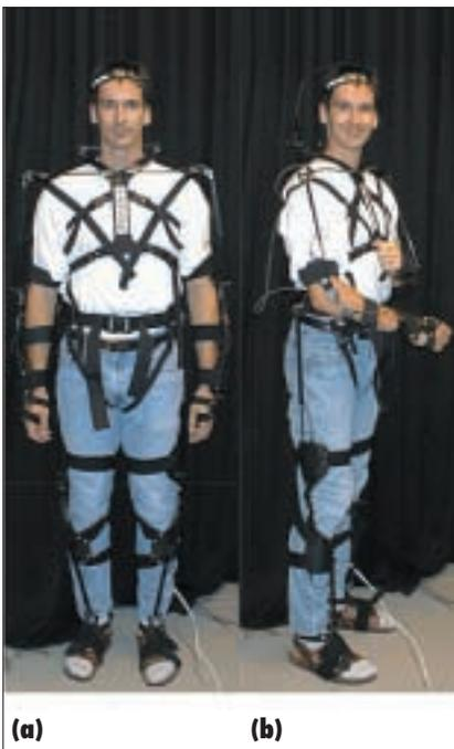
Figure 12. The Sensuit motion-capture system.
