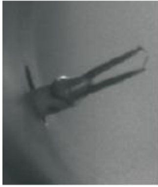
Fig. 3: The hooked hot-wire pushed into the gas passage.
