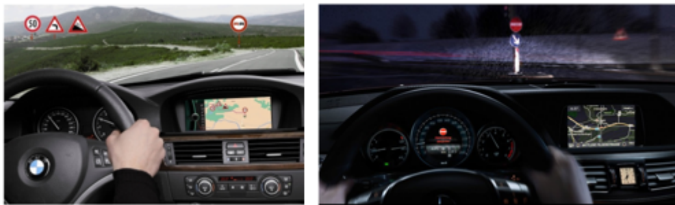
Figure 1.1: TSDR system on BMW heads-up display and Mercedes-Benz [2].
