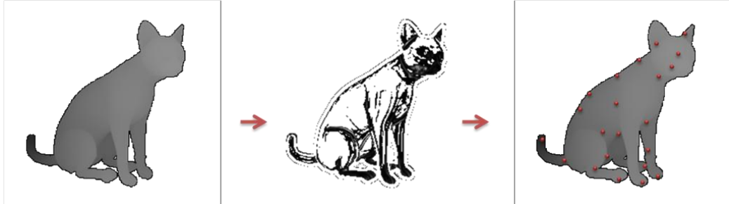
Figure 6-5 Keypoint selection, range image, surface variance mapping, keypoints as the maxima of the surface variance
