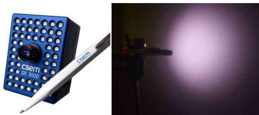
Figure 3-1. The CSEM SwissRanger SR3000 TOF Camera and its illumination. Second photograph is taken with a standard camera in night vision mode.
