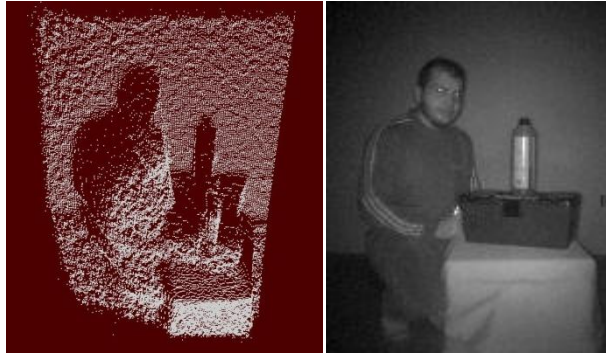
Figure 3-3. Point cloud and corresponding intensity image of the scene acquired by SR3000 TOF camera
