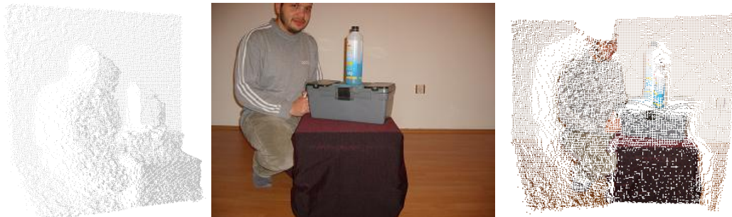
Figure 3-4. Point cloud obtained by TOF camera. Color image of the same scene acquired by a standard camera. Calibration of both images results colored point cloud data
