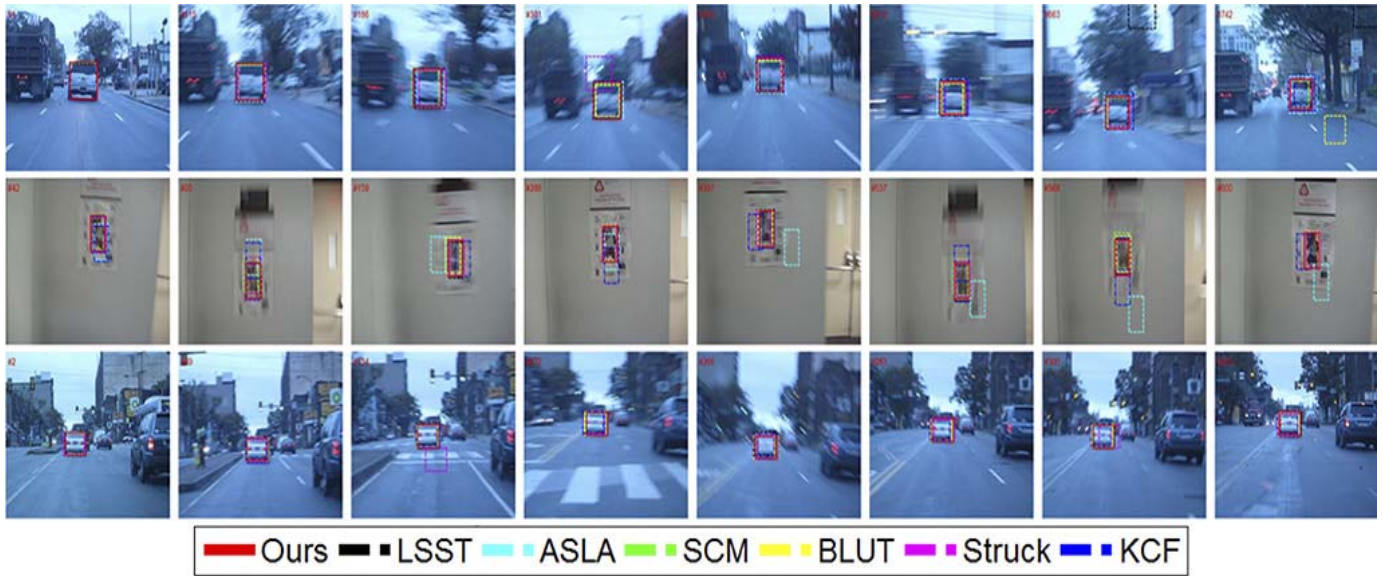
Fig. 2. Representative results of different trackers on sequences Car1 , Owl and Car3 . Objects in these sequences are under heavy motion blur.
