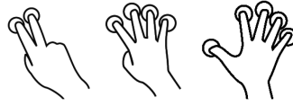
Fig. 3. A simple dissimilarity function for multi-touch gestures, inspired by the Finger-Count [8] technique, is the difference in the number of touches, e.g., \delta(\mathbf{p}_1, \mathbf{p}_2) = 2 , \delta(\mathbf{p}_1, \mathbf{p}_3) = 3 , and \delta(\mathbf{p}_2, \mathbf{p}_3) = 1 for the hand poses illustrated in this figure. However, for a tolerance of 2, transitivity is not met.
