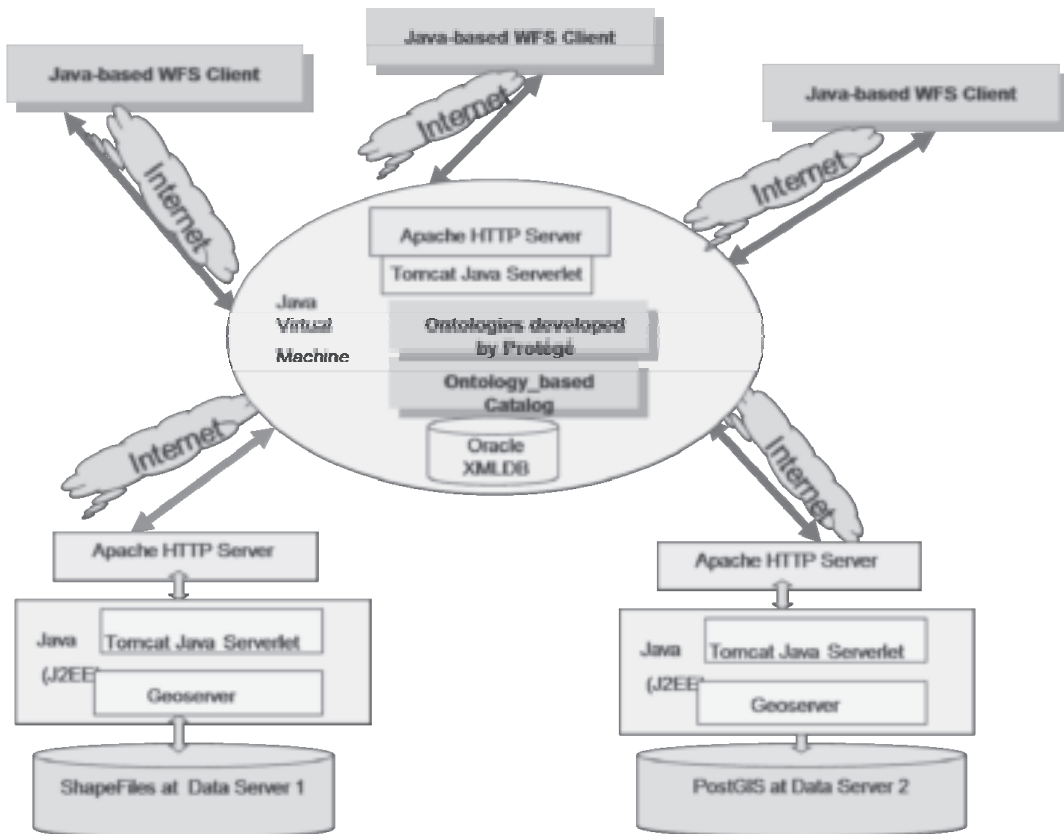
Figure 3. Architecture of the implemented prototype.
