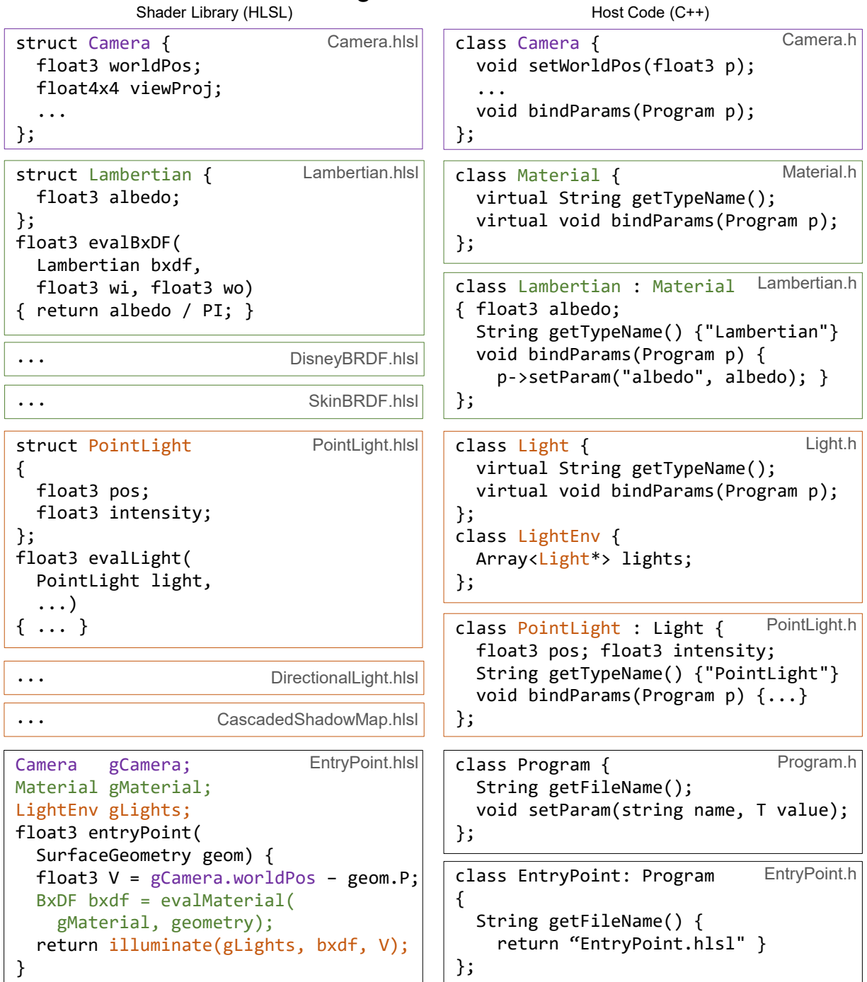
Figure 2.9: An example shading system architecture using HLSL and C++. The framework provides modules that comprise both HLSL struct types and corresponding C++ classes. The marshaling of data from CPU to GPU is managed explicitly by the bindParams methods on the C++ objects. A light type's evalLight function is called by the illuminate function, which is defined in Listing 2.3.
