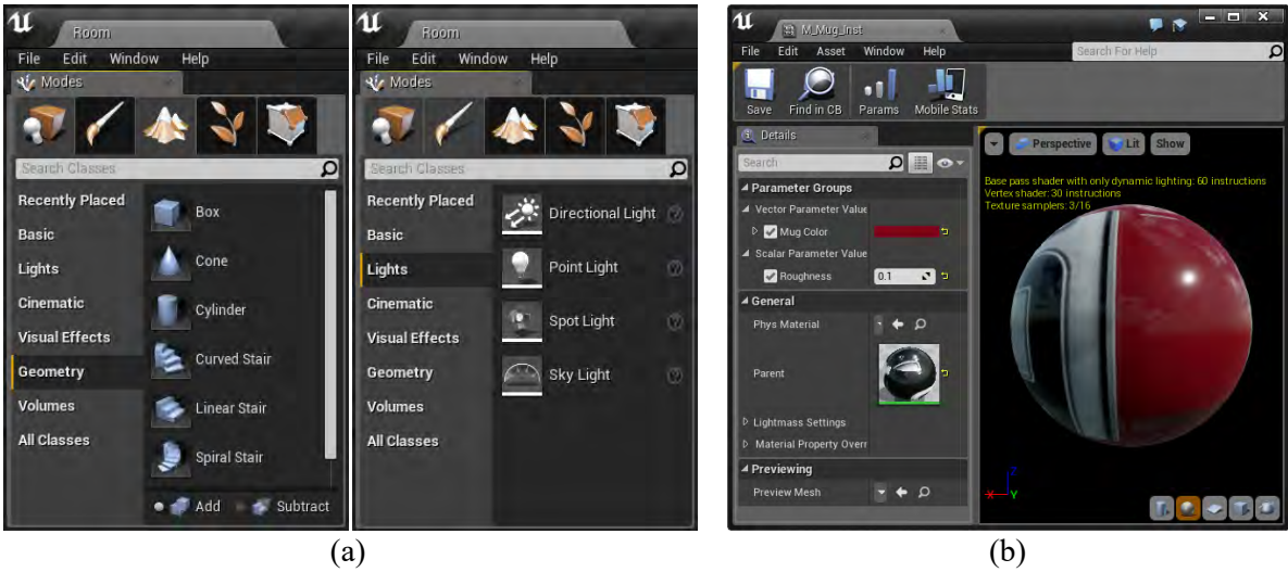
Figure 2.2: The GUI tools in Unreal Engine 4 reflects a typical graphics engineer’s mental decomposition for the shading problem. (a) Partial screenshots of Unreal Engine 4’s level editor show different types of geometry and lights. (b) Unreal Engine 4’s material editor allows a user to define object’s visual appearances.
