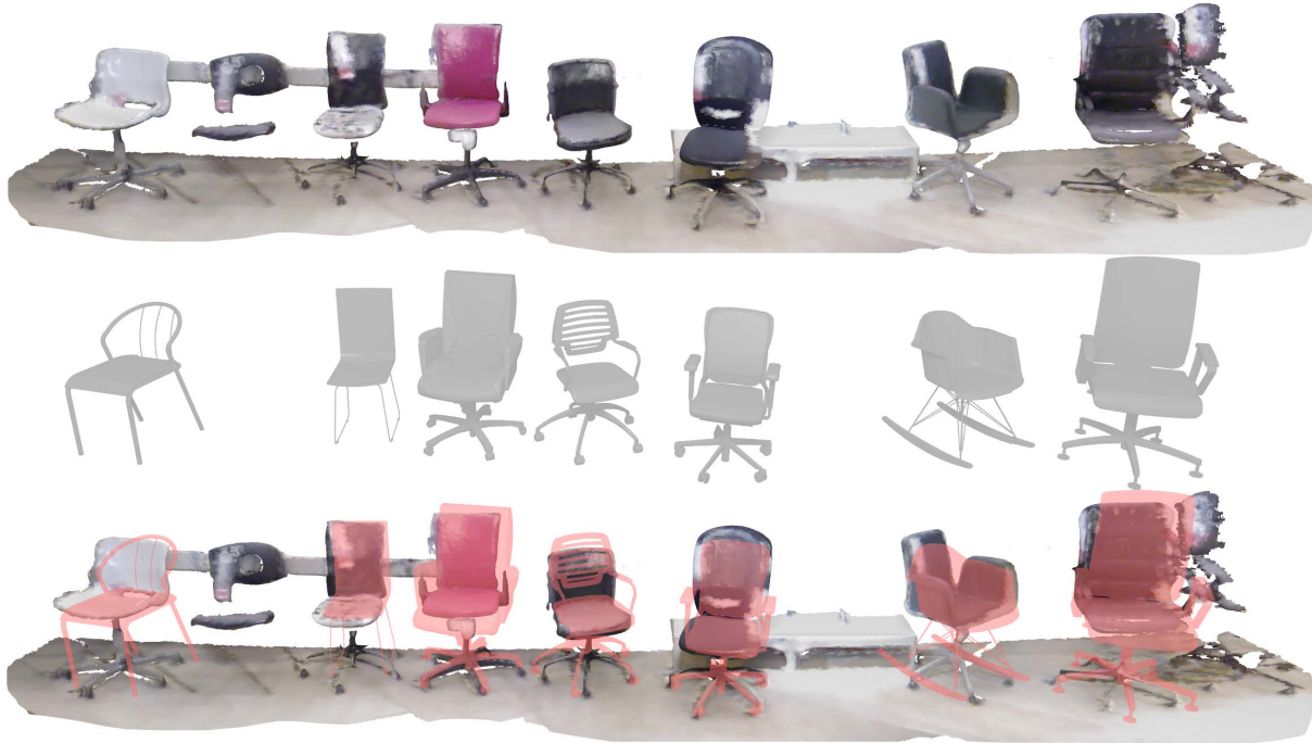
Figure 12: Results of our approach on a set of swivel chairs scanned at IKEA. The original 3D scan (top) is only a front view, including extremely partial coverage of the second chair from the left. Our object retrieval finds and registers very similar chairs for all but the very partially scanned chair (bottom), producing a clean, complete semantic reconstruction of the scene (middle).
