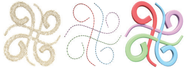
Figure 10: Since we represent cross-sectional profiles of arterial snakes using closed polyline-segments, our framework can naturally handle varying cross-sectional profiles. In this synthetically scanned dataset the gradually varying cross-sections (evolving from rectangle to circular profiles) are correctly identified.
