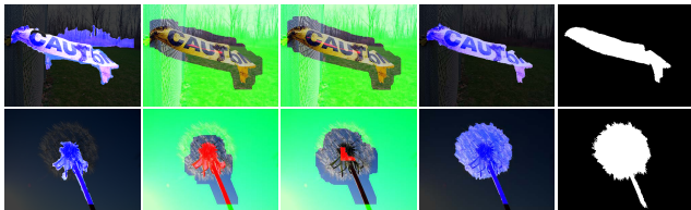
Figure 8. Saliency Cut. (Left to right) Initial segmentation, trimap after first iteration, trimap after second iteration, final segmentation, and manually labeled ground truth. In the segmented images, blue is foreground, gray is background, while in the trimaps, the foreground is red, the background is green, and unknown regions are left unchanged.
